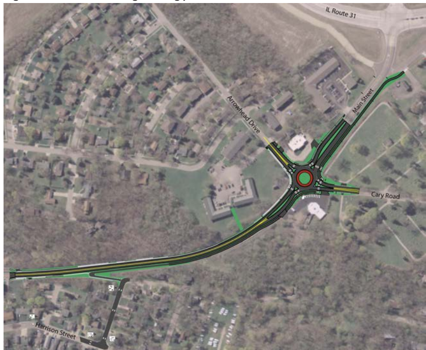
Figure 12. Roundabout engineering plan
